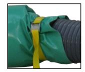
The other end of the flexible pipe can be fitted over the air outlet of the fan, it is held in place with a jubilee clip, which is tightened up using a flat-ended screwdriver. Do not over tighten as this may damage the pipe or the fan outlet.
