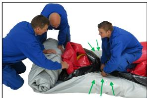
If the rolled unit is a bit loose or floppy unroll and do it again. When the unit is properly rolled up, tie it with the rope or strap provided.
