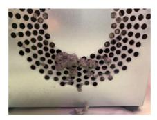
This is an example of just a few weeks of dust buildup. Already the fan will be working much harder to deliver the air. This can cause the fan to overheat and stop. If the fan cannot deliver the required air then the inflatable will be soft and potentially dangerous.
